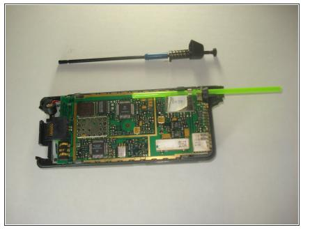
Slide the antenna out of the green tubing and slide the green tubing out of it's corresponding hole on the motherboard.
