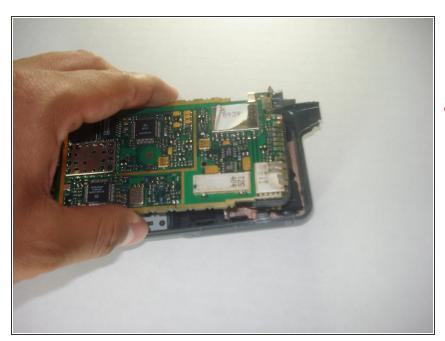
• Lift the motherboard out of its location in the front casing.
