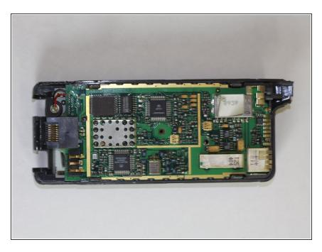
• Press firmly on the motherboard until it is snug inside the casing.
