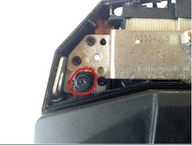
put back the black screws holding the front plate
