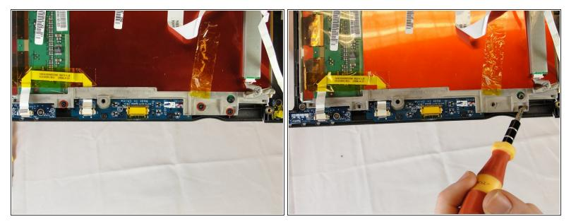
With a Phillips #1 screwdriver, unscrew the three 4mm screws holding the display bracket on the back side of the front buttons.
