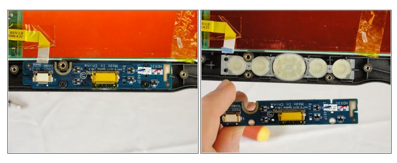
Remove the button board and replace.
