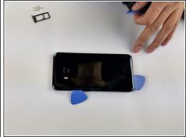
First, for easier opening, we need to heat up the mobile frame. Please be aware of the glass cracks while heating and opening.
