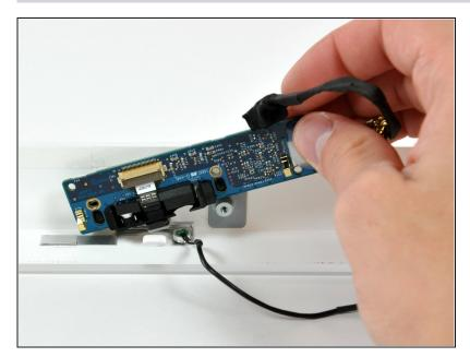
• Lift the camera board out from the front bezel.
