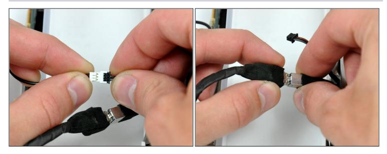
• Disconnect both the camera and microphone cables.
