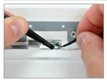
Use a spudger to pry the microphone off the adhesive holding it to the front bezel.
