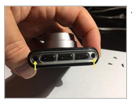
Remove the four case screws - 2 ea from the grey button panels using J000 phillips screwdriver bit
