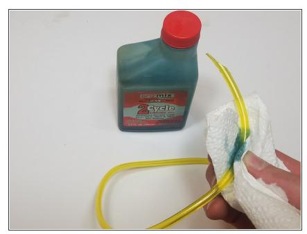
(i) Using 2-cycle oil as lubricant on the fuel lines will make it easier to pull them through the housing.
