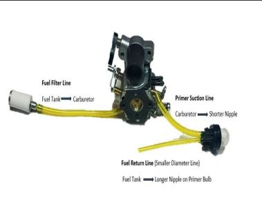
This is an example of how the fuel lines will attach to the carburetor and primer bulb.
