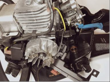
• Using a flat head screw driver or opening tool to disconnect the (primer-side) fuel line from the carburetor.
