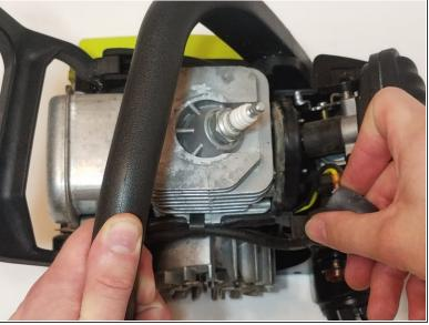
With the top cover off, disconnect the spark plug.
