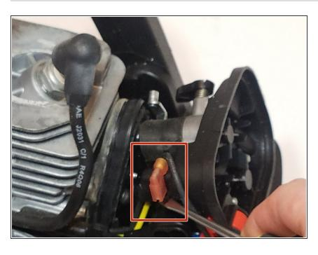
Use a spudger or flat head screwdriver to disconnect the kill switch wire.
