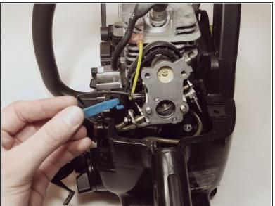
Remove the choke lever from the carburetor and set aside.
