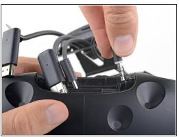
Repeat the lifting and unplugging process with the remaining USB, power, and audio cables.
