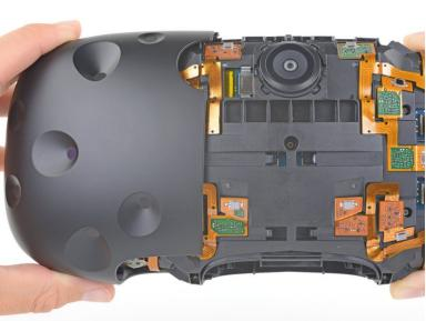
Repeat the last three steps for the left side of the outer shell and remove it.
