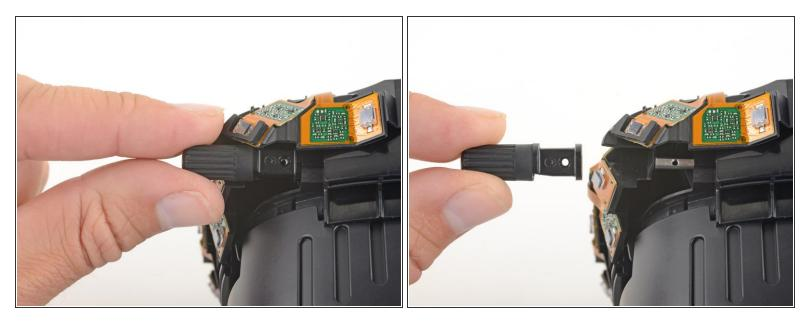
• Slide the focus knob off of the focus rod and remove it.
