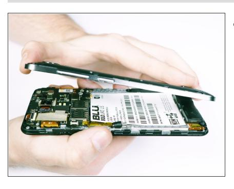
Once all the clips have been released, lift the frame and set it aside.
