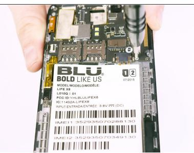
Use the Phillips #00 Phillips bit to undo the two 1.5mm screws from the motherboard.
