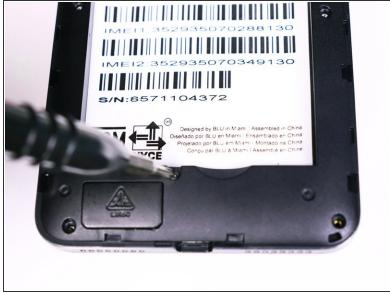
• Use the Phillips #00 bit to undo the nine 1.5mm screws from the back of the device.
