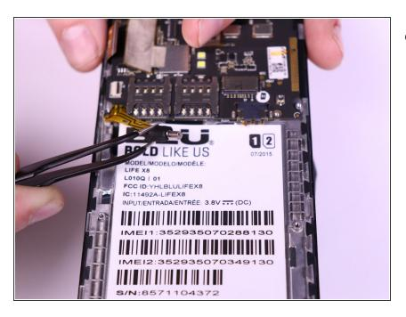
Slowly lift the vibration motor away from the frame and peel up the tape.
