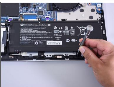
Use the Phillips Head 1 Screwdriver to remove the six 4 mm screws.
