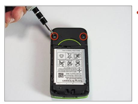
• Unscrew these two 5.4mm screws with a Torx T6 screwdriver.
