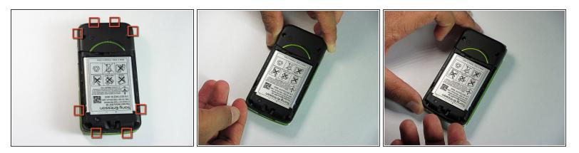
There are eight snap hooks located around the outer case. Carefully snap these to remove the outer case.
