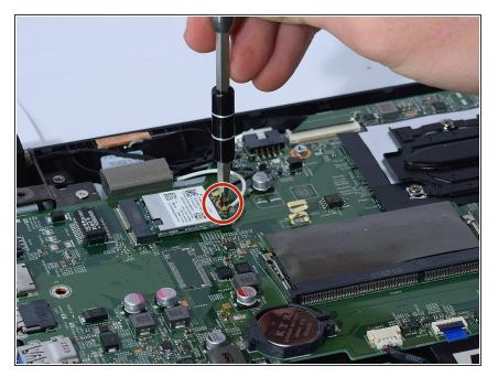
Remove single 3mm screw holding down the end of the card using a Phillips #1 screwdriver.
