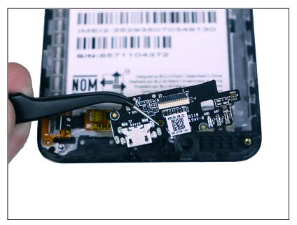
• Lift the daughterboard from the frame using the plastic opening tool.
