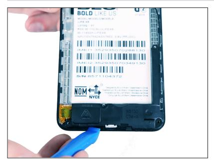
Use the plastic opening tool to pry off the plastic guard covering the daughterboard and USB port.
