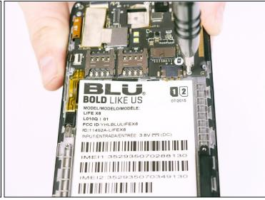
Use the Phillips #00 Phillips bit to undo the two 1.5mm screws from the motherboard.
