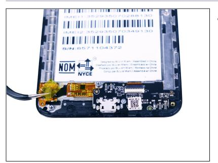
Remove the transparent tape covering one of the ribbon connectors using the <u>tweezers</u>.
