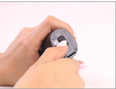
Open the battery compartment by locating the bottom of the handle, and pushing the slider forward.
