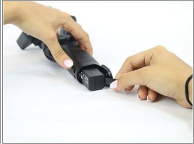
Take out the battery by pushing down on the red tab. The battery will release, and can be pulled out by using the attached black tab. To reassemble your device, insert the new battery and follow these instructions in reverse order.
