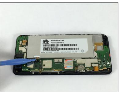
Use a plastic opening tool to remove the pictured flat-top connector.
