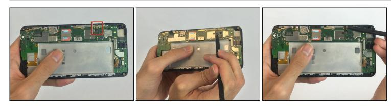
• Using the spudger, pry open the zif connector, and remove the cable.
