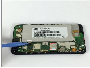
Use a plastic opening tool to remove the pictured flat-top connector.
