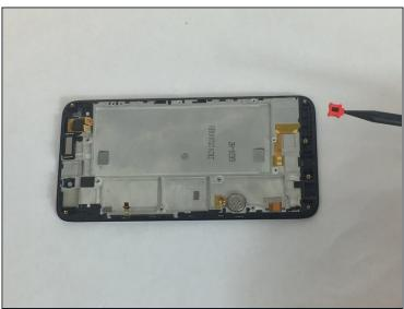
• Using <u>tweezers</u> or the spudger, remove the microphone.
