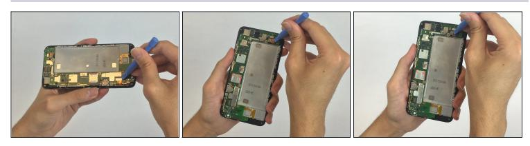
• Use the plastic opening tool to remove all the remaining flat-top connectors.
