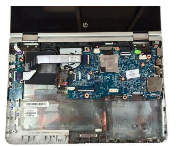
Holding the lower right corner, gently lift up the battery to disconnect it from the motherboard.
