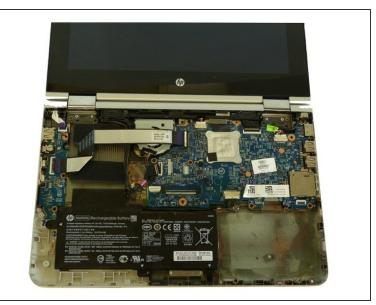
After the ribbon cables are disconnected, gently lift up the keyboard to disconnect it from the base of the laptop.
