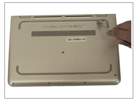
Flip the laptop over and remove the rubber foot with a Metal Spudger.
