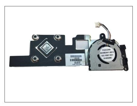
Disconnect the fan from the motherboard by taking out the screws.
