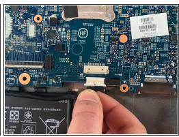
• Disconnect the 3 bundle cable connectors by gently gripping the cable wires and pulling outwards.
