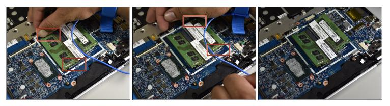
• Pull the two outer pins on either side of the ram chip outward with your hands.
