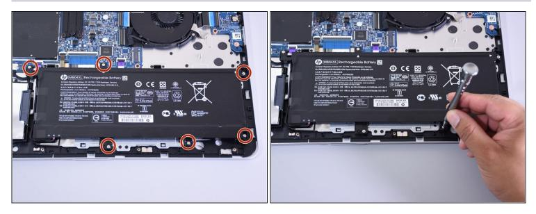
• Use the Phillips Head 1 Screwdriver to remove the six 4 mm screws.
