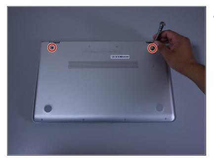
• Remove the two 8 mm Phillips Head screws that were under the grip pads using a Phillip's Head 1 Screwdriver.
