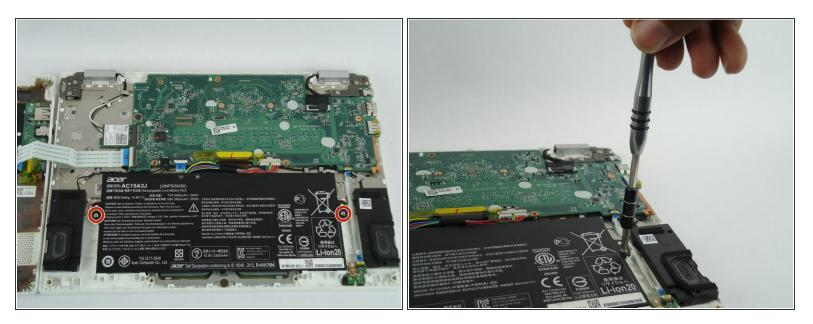
• Unscrew the (2) two 3mm J0 Phillips head screws that hold the battery in place.
