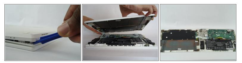
• Use the plastic opening tool to remove the back cover.
