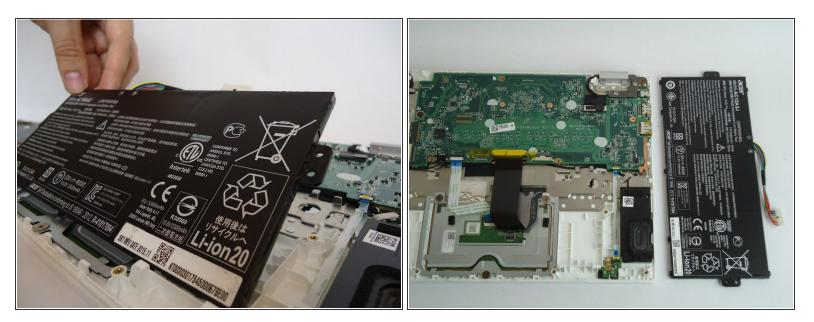
• Carefully lift the battery from one side, and then lift it out of the laptop.
