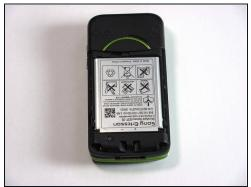
Unscrew the bottom two 5.4mm screws with a Torx T6 screwdriver.
