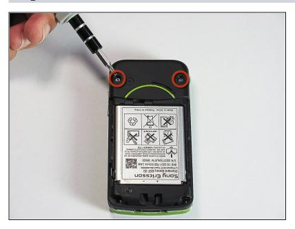
Unscrew these two 5.4mm screws with a Torx T6 screwdriver.
