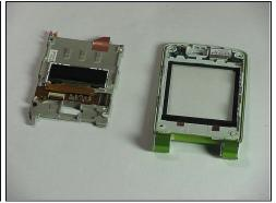
• Pull apart the screen and the case at one end. Then slide the screen out to completely detach them.
