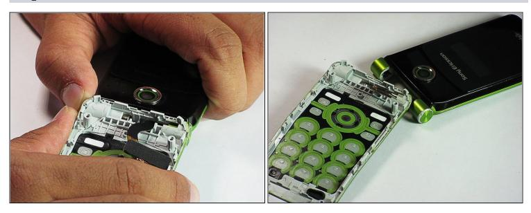
• Separate the bottom and top half of the phone from the hinge they are connected by.
