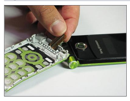
Pull the ribbon through the opening in the hinge to completely separate the upper and lower halves of the phone.
