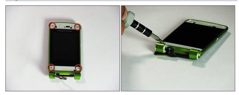
• Remove the four 5.4 mm screws with a Torx T5 screwdriver.
