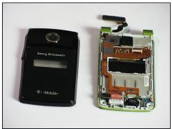
Use a plastic opening tool in the indicated location and apply pressure until the case hook is detached. Then lift the case up until the two pieces are detached.
