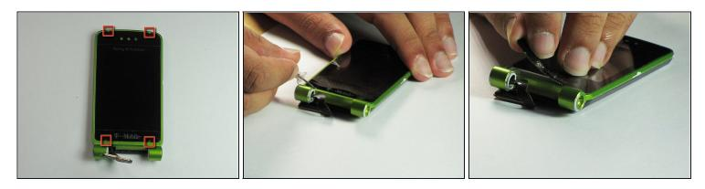
• The top and bottom covers are held in place by adhesive. To remove them, use a pushpin in the four indentations indicated to remove.
