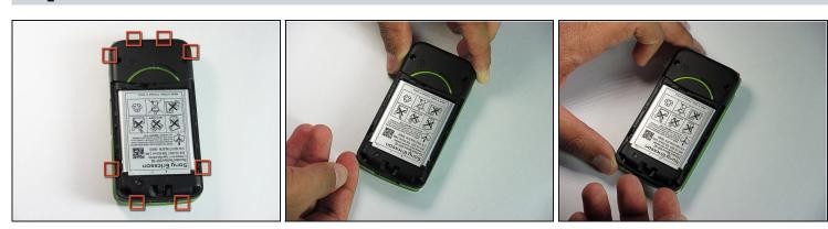
• There are eight snap hooks located around the outer case. Carefully snap these to remove the outer case.
