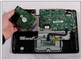
• Locate the hard drive and slide the hard drive to the left until it disconnects from the mother board.
