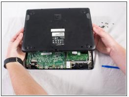
• Using a plastic opening tool, gently pry the lower case off. Place aside.
