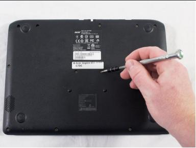
Unscrew the 13 6.2mm screws located on the bottom of the laptop using the JIS #0 screwdriver.
