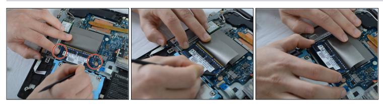
• Push outwards on the metal tabs located on both sides of the RAM to release the RAM. You can use the spudger tool if you have any issues.
