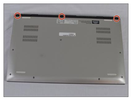
Use the screwdriver to take out the three 5mm black JIS #1 head screws that are located on the hinge.
