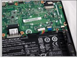
Using your fingers or the small plastic opening tools, disconnect the battery connection from the motherboard by pinching and pulling back on both sides of the connector.
