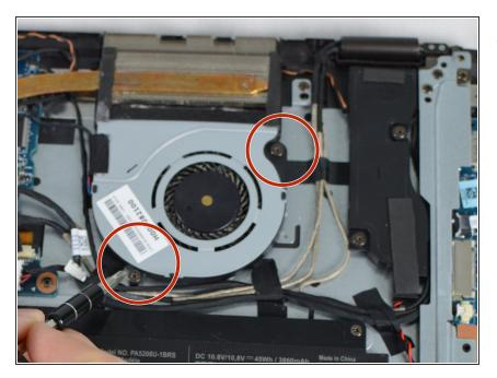
Unscrew the two 7 mm JIS #1 head screws securing the fan to the laptop.
