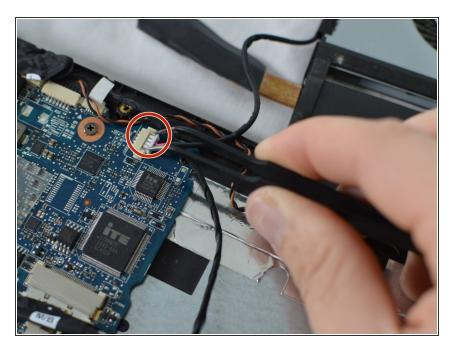
Using tweezers, disconnect power cable by gently pulling white end out from its socket.
