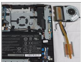
Based on the quality of the fan either the clean fan or replace the fan.
