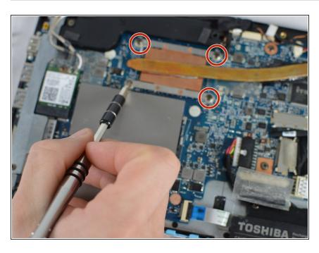
Remove heat sink by unscrewing the four 3 mm JIS #1 head screws
