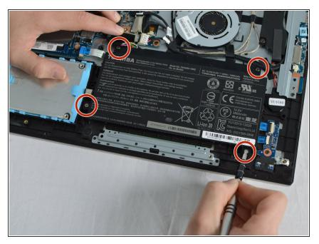
Unscrew the four 5 mm JIS #1 head screws holding the battery to the device and gently remove the battery.
