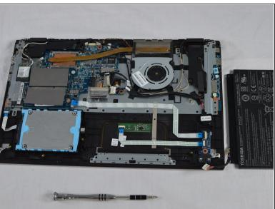
Disconnect the battery from the motherboard by gently pulling out the black connector.
