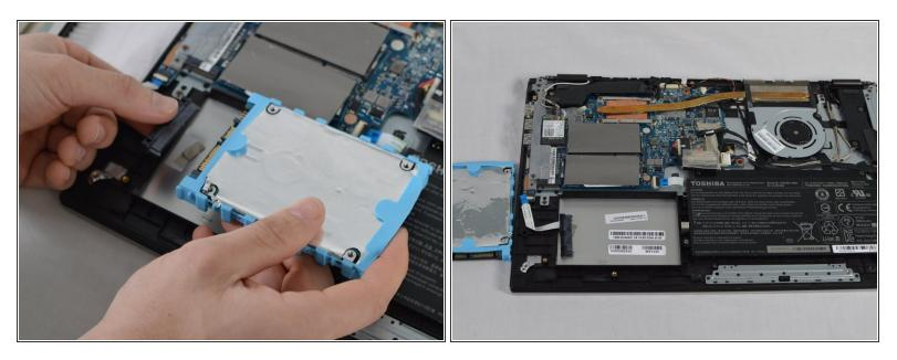
• Disconnect the hard drive from the mother board by gently pulling out the black connector.
