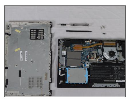
• Remove the back cover of the device.
