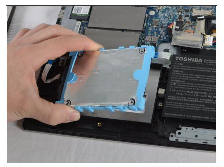
Remove the hard drive from the device by gently pulling on the blue plastic hard drive cover.
