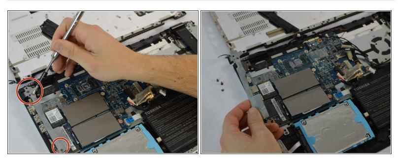
Remove all three 5 mm silver JIS head screws connecting the silver cover to the motherboard.
