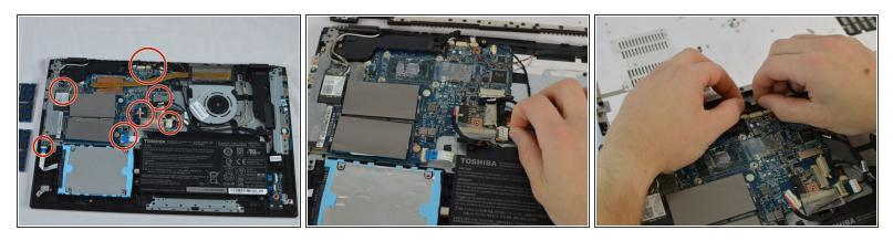
Remove all power connections to the motherboard. Including the black and white power connections to the wifi module.
