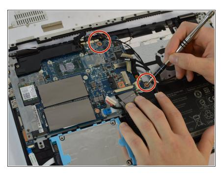
Remove both 3mm JIS head screws connecting the motherboard to the device.
