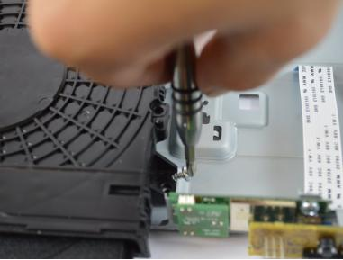
Remove the two screws that attach the disk drive to the frame using a #1 Phillips screwdriver.
