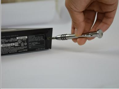
Use a #1 Phillips screwdriver to remove the three screws located in the back of the device.
