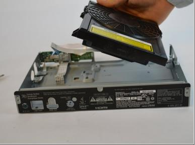
• Lift the disk drive off of the device
