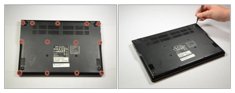
Use a Phillips head screw driver to remove the 13 screws in these locations.
