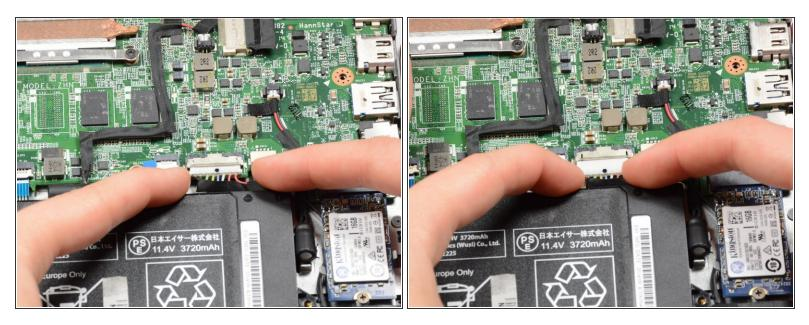
• Use two fingers to unplug the battery-to-motherboard connection.
