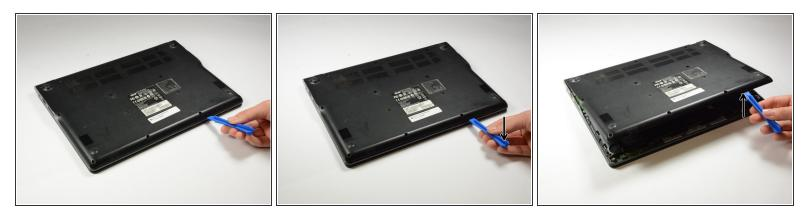
• Use a plastic spudger to pry up the bottom cover and remove it.
