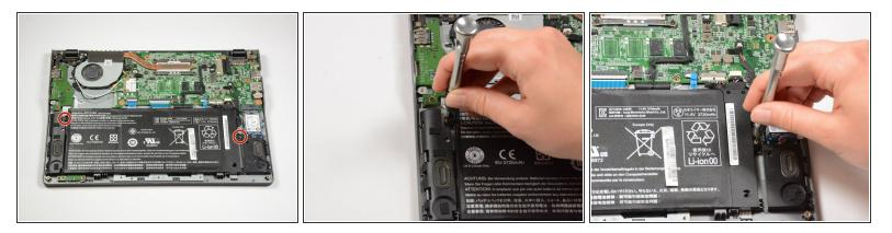
Unscrew the 2 battery screws.
