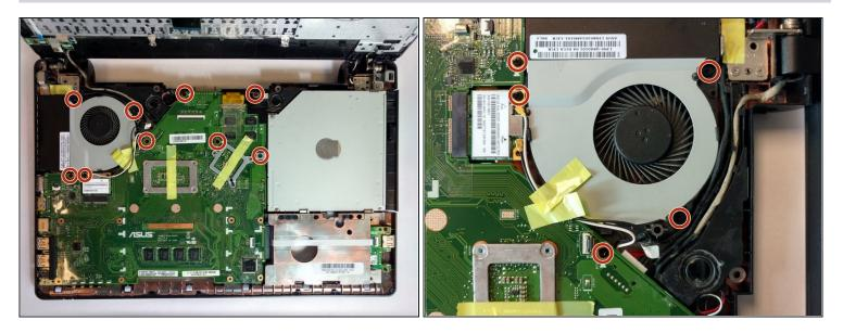
• Using the Phillips #0 Screwdriver, remove the nine 2mm screws at the marked locations.
