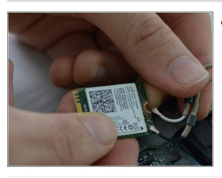
Remove the black and white wires that are connected to the device by gently pulling on it.
