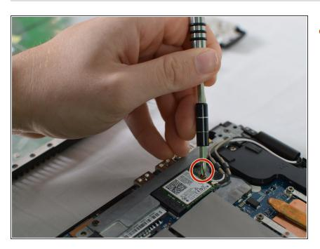
Unscrew the 3mm JIS head screw with J1#1. This screw is holding the Wi-Fi module to the device
