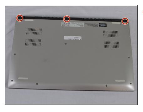
Use the screwdriver to take out the three 5mm black JIS #1 head screws that are located on the hinge.
