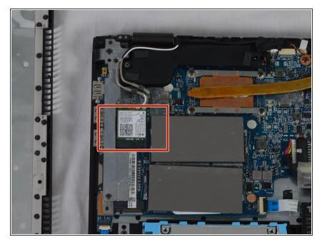
Locate the Wi-Fi module in the device which is located next to the ram.
