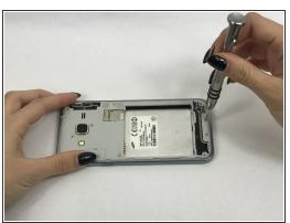
Remove the ten 2.0 mm screws with the Phillips #J000 screwdriver.
