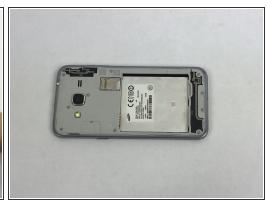
Place your thumb on the top left corner and pry the tab open and lift off the back cover.
