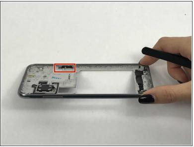
• After opening the phone, locate the power button on the back frame of the phone.
