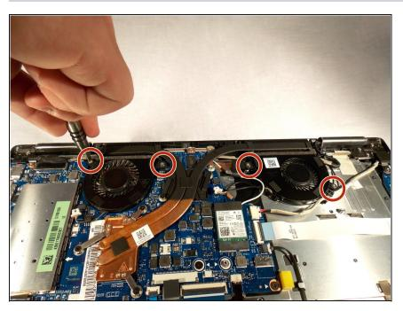
Use a Phillips #1 screwdriver to remove the four screws holding down the fans.
