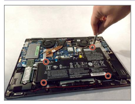
Remove the four 3.5 mm screws around the battery using a Phillips #1 screwdriver.
