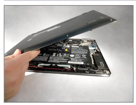
• Lift and remove the back cover.
