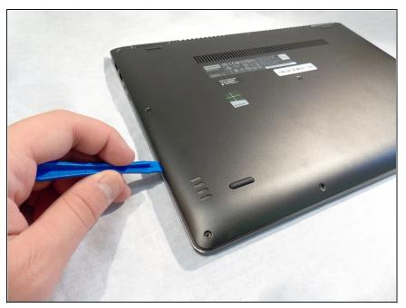
Slide an opening tool between the base and back cover and work your way around the entire device to release the back cover.
