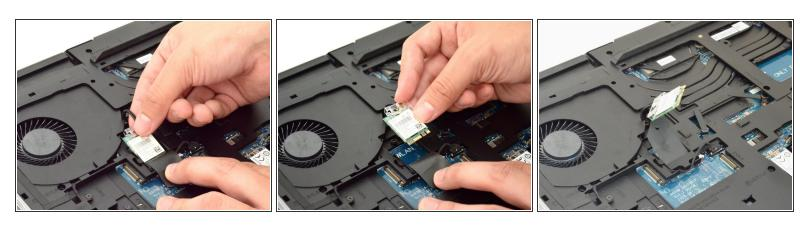
Gently undo the clips attached to the wi-fi card.
