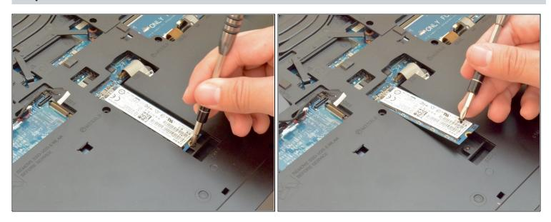
• Remove the one M2x3 screw (1.9 mm) using a PH1 screwdriver bit
