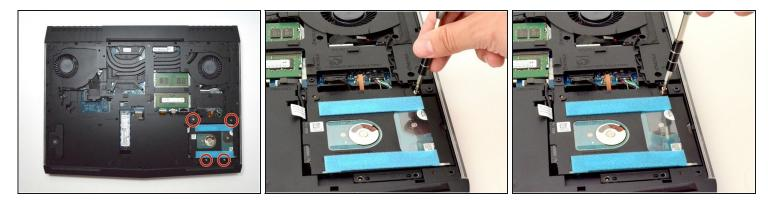
Use a PH1 screwdriver bit to remove the four M2.5x5 screws (2.4 mm) on the hard disk drive.
