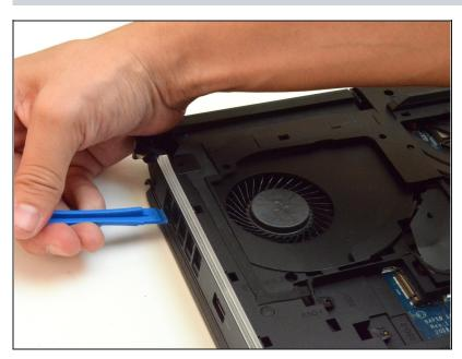
• Use the **plastic opening tool** to gently lift the sides of the cover.
