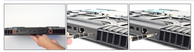
Remove the two M2.5x7 screws (2.44 mm) located on the rear panel using a PH1 screwdriver bit.
