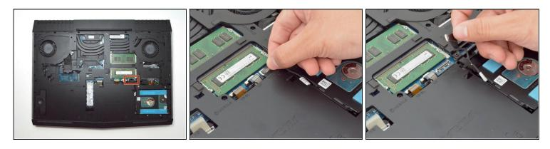
• **Gently** lift the HDD cable to disconnect it from the laptop.
