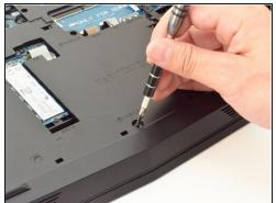
Remove the fourteen M2.5XL8' screws (2.4 mm) located in the plastic cover using the PH1 screwdriver.
