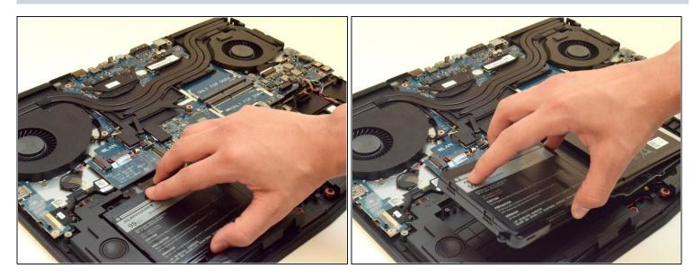
Lift the battery up to remove it.
