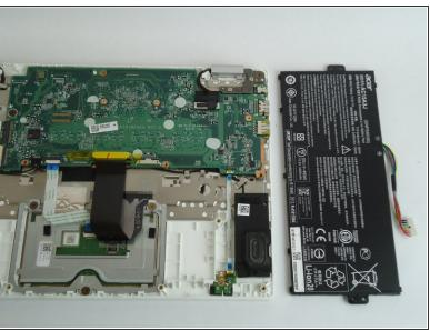
Carefully lift the battery from one side, and then lift it out of the laptop.
