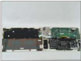
Use the plastic opening tool to remove the back cover.
