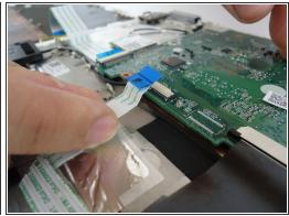
• Disconnect the three ribbon cables from the motherboard.
