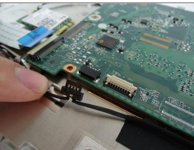
Unplug the cable by putting both thumbs on each tab and unlocking the cable by pushing the tabs away.
