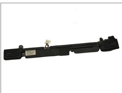
After the screws are out, lift out the speaker from the base of the laptop.
