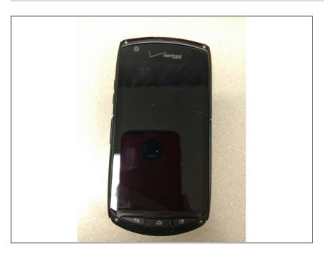
Remove the four screws, one in each corner. Use a Y0 screwdriver bit.
