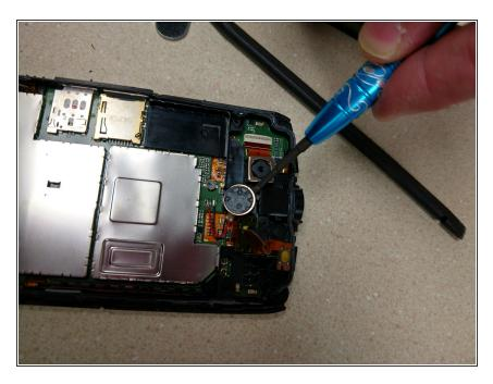
Lift the vibrate motor out. It is held in by some mild adhesive.
