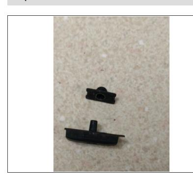
Each button has a rubber grommet over the inside to keep it water resistant. Be sure to remove those if they don't pop out with the buttons, setting them aside together for reassembly.
