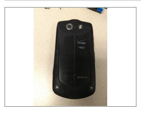
The two silver screws at the bottom of the back plate are decorative and cannot be removed from here.
