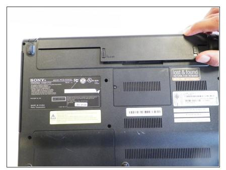
Unlock the battery by sliding the lock upwards.
