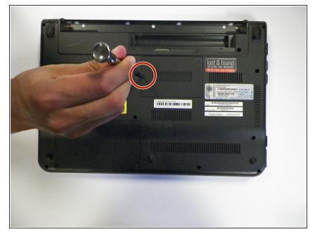
Use a Phillips #1 screw to unscrew the 6.5 mm screw keeping the cover.
