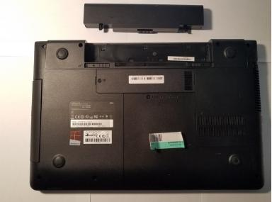
Press and pull the two battery locks in the outward direction and pull the battery out. And then new battery can be replaced.
