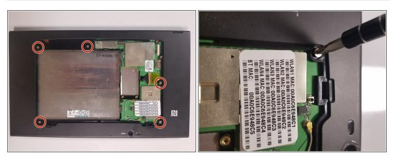
Use the Phillips PH1 screwdriver to unscrew the five 4x2.5mm screws that hold the back cover.
