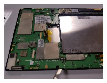
• Using the spudger lift the motherboard out of the tablet frame.
