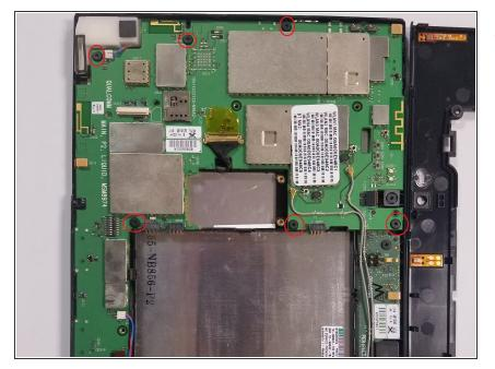
Using the Phillips PH1, remove all 6 of the 3x2.5mm screws (circled in red) holding the motherboard in place.
