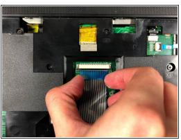
Once the keyboard is free, disconnect the ribbon cable from the zero insertion force (ZIF)
