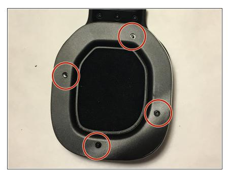
Remove the four 3.5mm Phillips head screws circled in red, and remove the grey cover.
