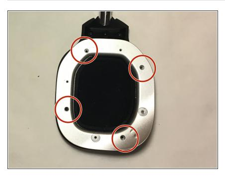
Remove the four 3.5mm Phillips head screws circled in red and remove the silver cover.
