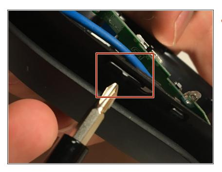
Finally push the channel selector in towards the motherboard to remove it from the headset casing. The switch is pointed to by the screwdriver inside the red square.
