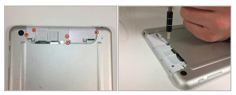
Using the Phillips Head #000, unscrew the 5 4mm and 3mm screws at the top.
