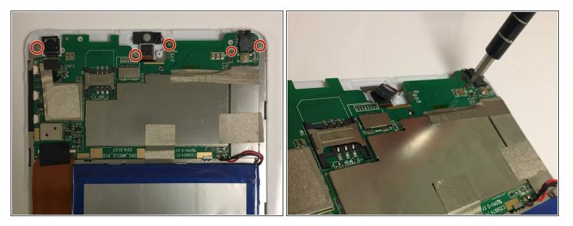
Unscrew 5 #000 4 mm and 3 mm screws around the strip.
