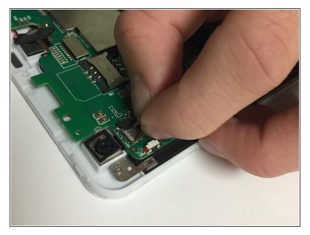
Undo the tape on top of the connector from the camera to motherboard.
