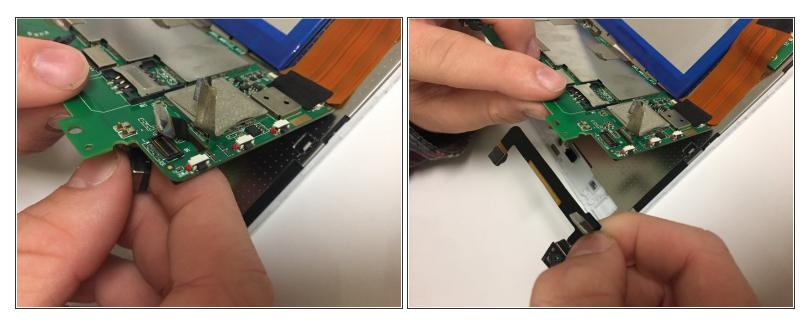
• Disconnect the camera from the motherboard on the topside and pull the camera strip out.
