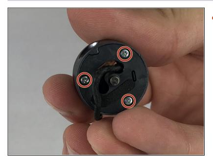
Remove the three 5mm screws holding together the camera housing using a PH00 screwdriver.
