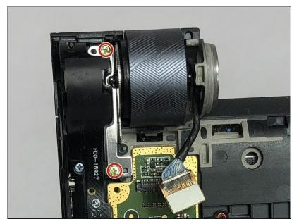
Locate the silver camera mounting bracket between the power button and the camera housing. Remove the two 3mm screws on the camera mounting bracket using a PH00 screwdriver.
