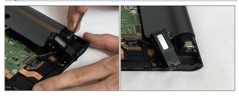
• Position the kickstand to an almost closed position. Carefully move the plastic block aside and pry the metal lock out with a metal spudger.
