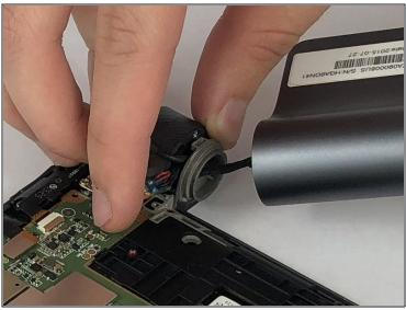
• Begin removing the entire hinge assembly by lifting it out, starting at the end where the lock is located. Carefully feed the wires through the hinge mount with your fingers as you pull the hinge assembly free.
