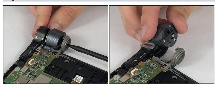
• The camera housing is held in place by a pin in the center of the grey hinge mount. Push and hold in the pin with the pointy end of a spudger while you lift the camera assembly out.
