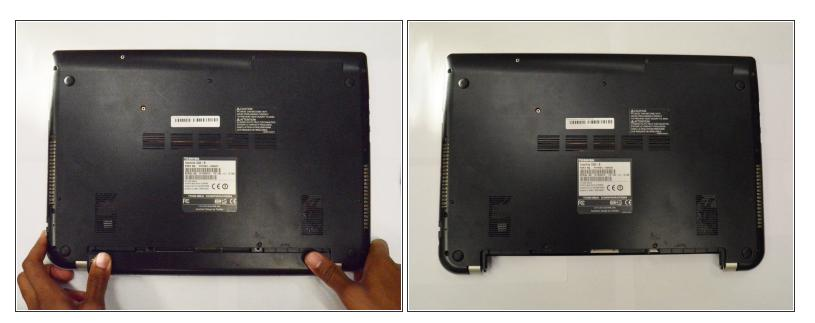
Place thumbs on corners of the battery. Pinch the battery between the thumb and index finger and pull.
