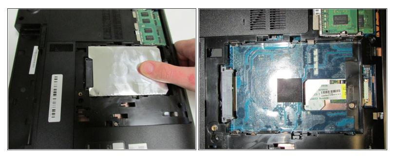
• To remove the hard drive, use a small amount of force and slide it out.
