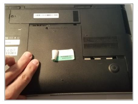
Using your hand slide the ODD/HDD/Memory panel off in a downward motion.
