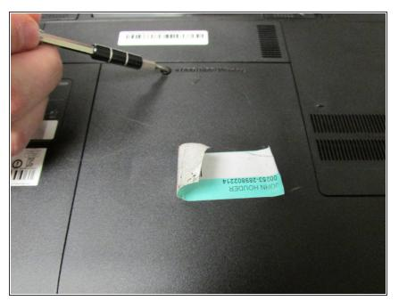
• Using the Phillips #1 screwdriver, remove the M2.5X5 mm screw to take the back cover out.
